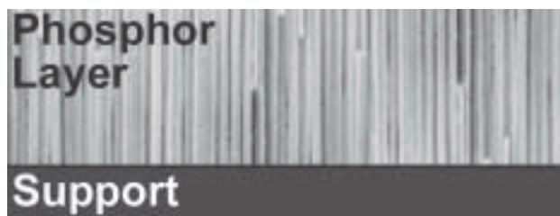
Figure 13. Cross-section of a structured SP screen showing the needlelike storage phosphor rods perpendicular to the substrate. The substrate can be either opaque or transparent, depending on the application and the desired scanning geometry. As with powder SP screens (Fig 5), additional layers are needed to optimize performance.
