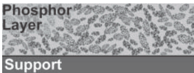
Figure 5. Cross-section of a prototypic storage phosphor screen showing the two main layers (active phosphor and support). A number of other (manufacturer-dependent) layers are added to optimize the mechanical, optical, and electrical performance of the screen.
