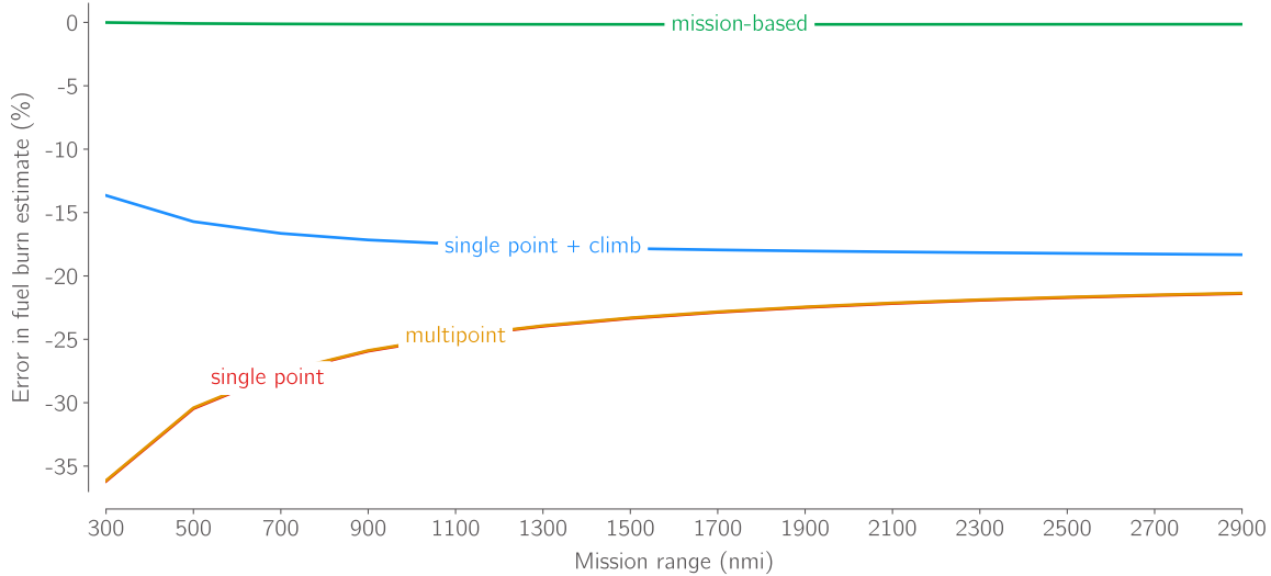
Fig. 15 The new method better approximates the true fuel burn compared to single point. For this figure, a fuel burn estimation in descent for single point + climb is included for a fair comparison between the methods.
