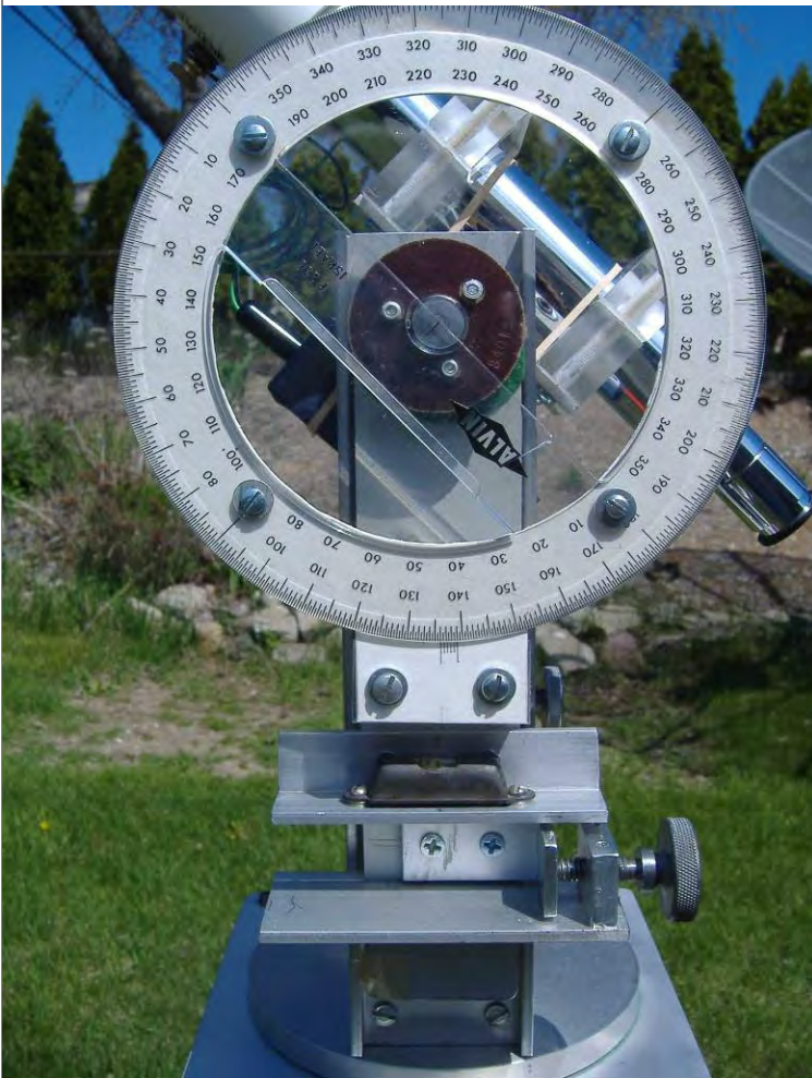
Figure 2 Close-Up Showing Vernier Dial and Spirit Level
