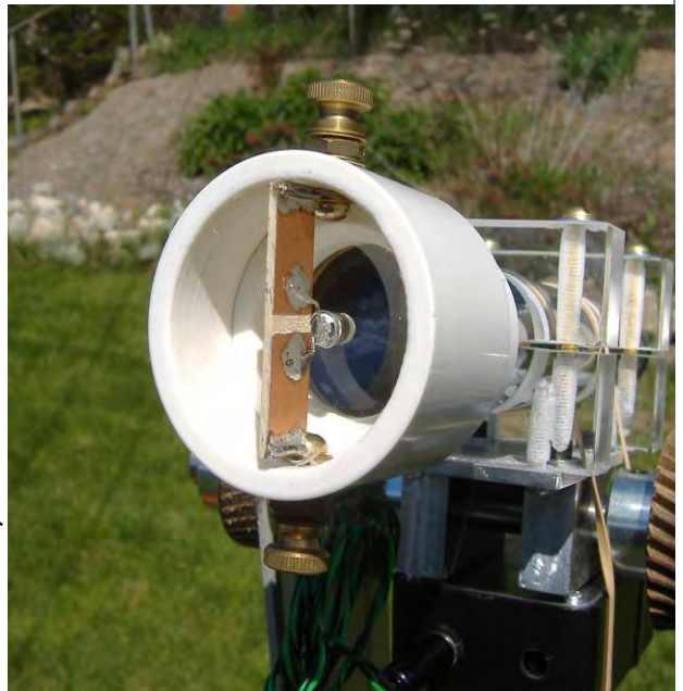
Figure 3 LED Background Illumination Attachment
