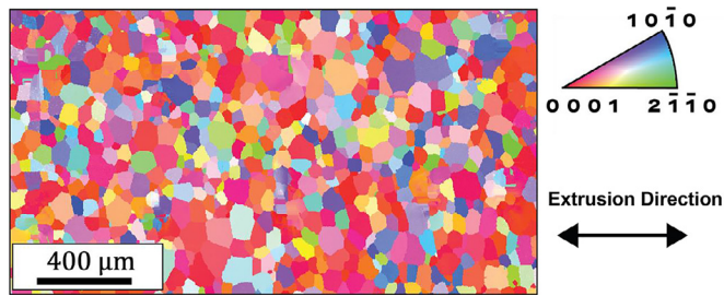
Fig. 2. EBSD inverse pole figure map of extruded Mg-4Al (wt.%) with the average grain size of 55 \mu\text{m} .
