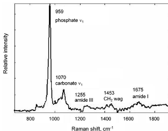
**FIG. 2.** Raman spectrum of a 6-month-old WT mouse femur. Important bands discussed in this paper are indicated together with their vibrational assignments. The amide II,  $\text{CH}_2$  wag, and amide I bands result from vibrations of the collagenous matrix, whereas the phosphate  $\nu_1$  and carbonate  $\nu_1$  bands arise from the bone mineral.
