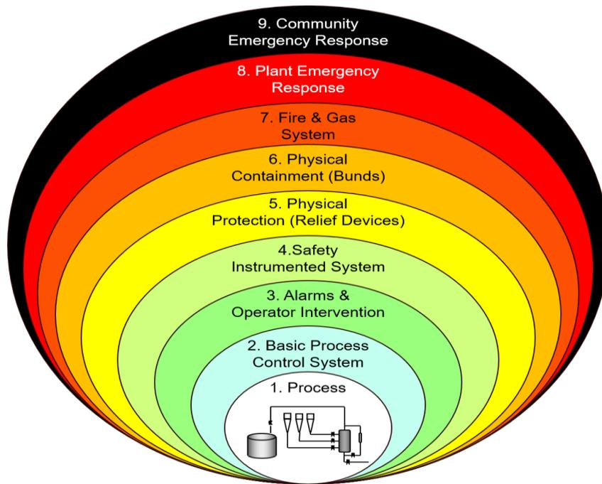
Figure 1. Layers of Protection Example Visual [5]
