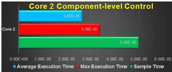
Fig. 17. Real-time simulation evaluation of component-level controllers (core2).
