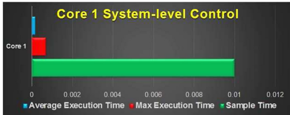
Fig. 16. Real-time simulation evaluation of system-level controller (core1).
