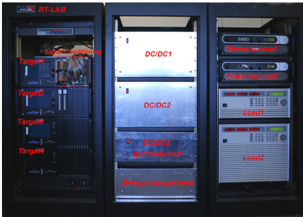
Fig. 6. Scaled test bed of HPS [23].
