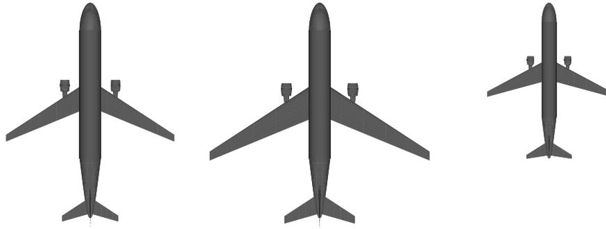
Figure 2. Planform view of LASR (left), A330 (center) and A320 (right)
