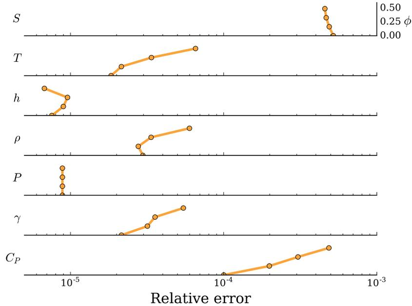
Fig. 8: Mean relative errors between the thermodynamic states predicted by CEA and by proposed code is less than 0.1%.
