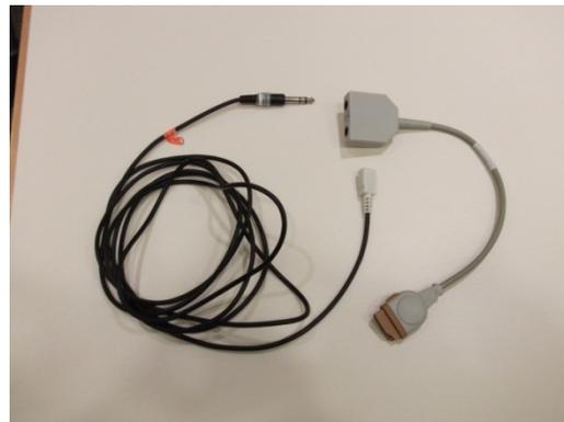
**Figure C-6: Temp Sensing Cable**
