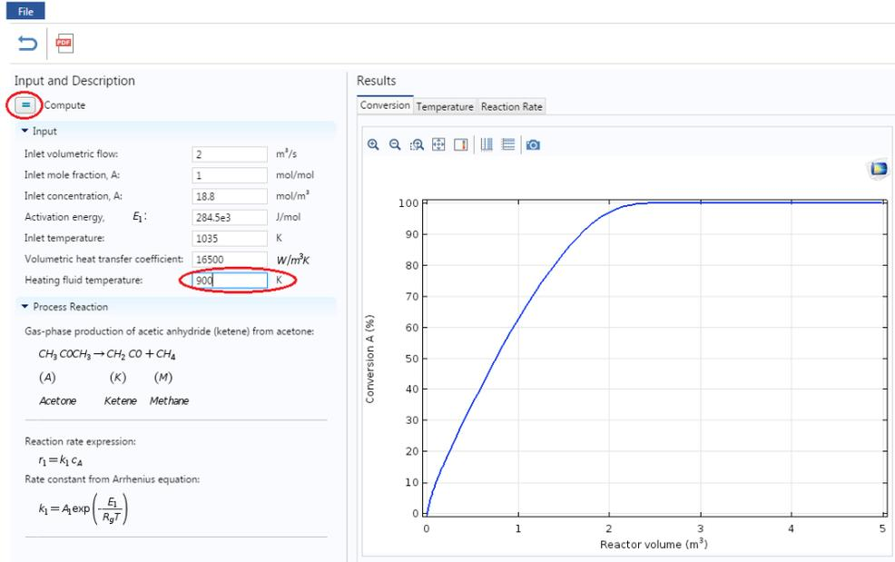
**Step 8:** Now check the Conversion and Temperature profiles. The following graph is obtained for Conversion. You can see that conversion has decreased at lower heating fluid temperature
