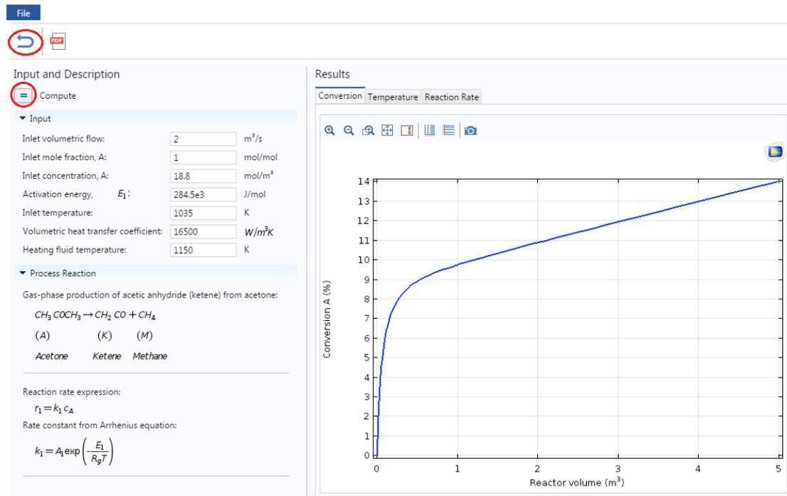
**Step 10:** Now let's consider a case where you want to maintain the Inlet concentration such that 100 % conversion is achieved at the end of the reactor. Enter the inlet concentration of A as 50 mol/m<sup>3</sup> and click compute to see its effect on profile.
