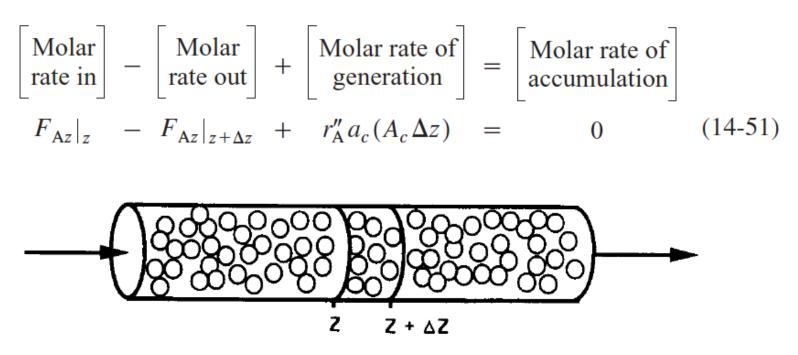
Figure 14-5 Packed-bed reactor.
