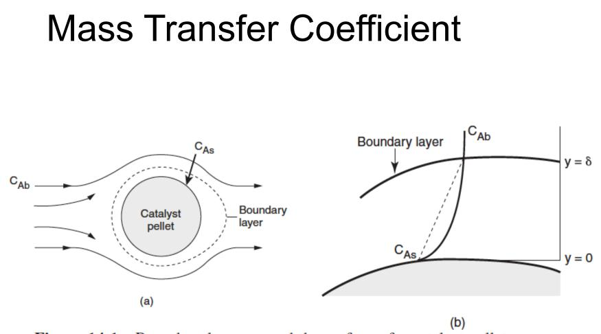
Figure 14-1 Boundary layer around the surface of a catalyst pellet.
