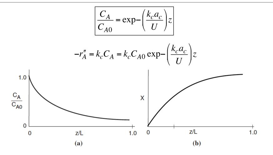
Figure 14-7 Axial concentration (a) and conversion (b) profiles in a packed bed.
