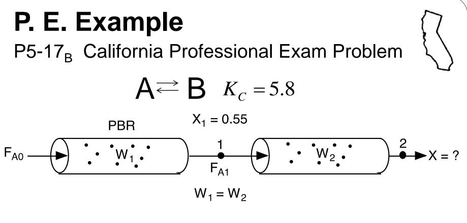
$X_2 = \frac{\text{Total moles reacted at Point 2}}{\text{Mole fed to first reactor}}$
