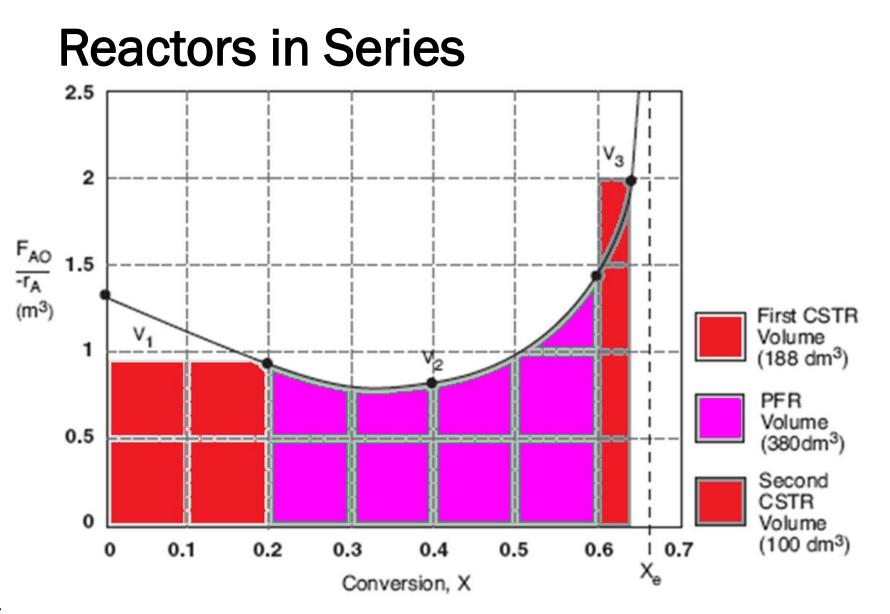
Space time  $\tau$  is the time necessary to process 1 reactor volume of fluid at entrance conditions.
