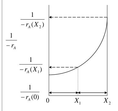
$$V = \int_{0}^{X} \frac{F_{A0}}{-r_{A}} dX = \frac{\Delta x}{3} F_{A0} \left[ \frac{1}{-r_{A}(0)} + \frac{4}{-r_{A}(X/2)} + \frac{1}{-r_{A}(X/2)} \right]$$
