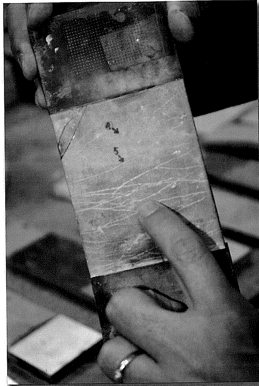
The white lines on this specimen of bendable concrete show where the material has healed itself by forming \text{CaCO}_3 . This specimen has undergone deliberately introduced damage and succeeding self healing numerous times, illustrating the resiliency necessary for field structures that may undergo multiple overloads during their lifetime. Photo by Nicole Casal Moore, University of Michigan News Service.
